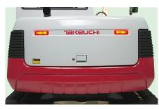
\*REAR MOUNTED WORK LIGHTS improve job site safety conditions by visually alerting anyone entering the excavators
