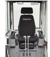
MULTI-ADJUSTABLE SUSPENSION SEAT provides for long days productive operation with minimal operator fatique
