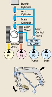
The optimal combination of high digging forces and fast cycle times are continuously adjusted according to the variable digging loads encountered by the excavators.
